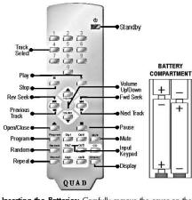
Inserting the Batteries: Carefully remove the cover on the rear of the handset. Unwrap the four supplied AAA batteries and insert them in the positions shown. Replace the cover.
