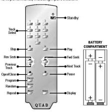
Inserting the Batteries: Carefully remove the cover on the rear of the handset. Unwrap the four supplied AAA batteries and insert them in the positions shown. Replace the cover.
